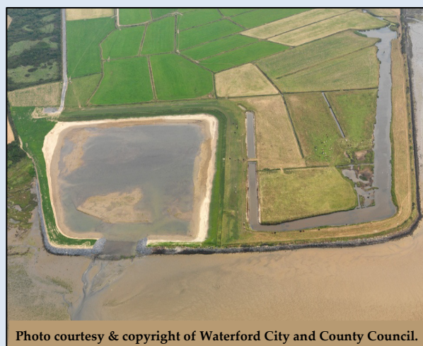
Figure 5. Aerial views of the MR site at Kilmaclegue West dated 2004 (left) and c. 2013 (right). The newly inundated area, new levee and the breach in the old levee can be seen on the left of the photo taken c. 2013.
